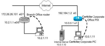
Assignment: Click on the picture of the host connected to an IDS Sensor by a serial console cable shown in the diagram as a dotted line. Select the Cisco Terminal Option and make the appropriate configuration tasks.
